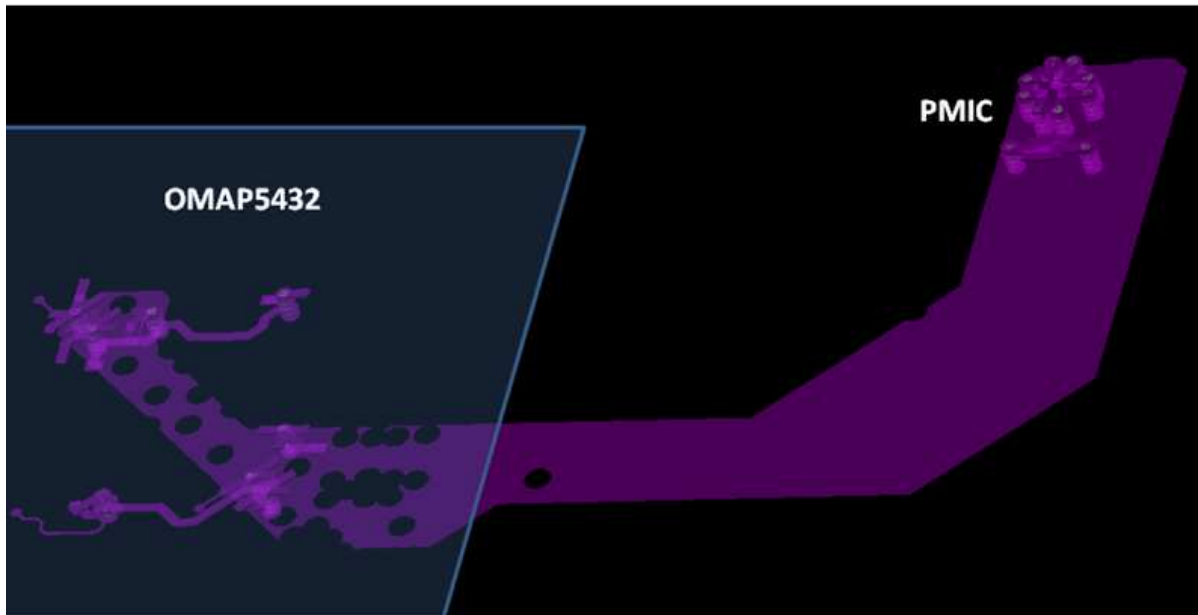
Figure 7-24. vdd_mm PCB Routing (1)
