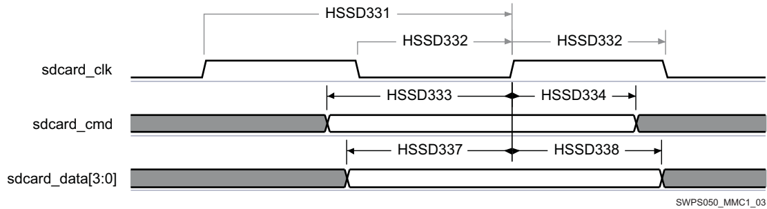
Figure 6-92. High Speed SD Card, 3.3 V—Receiver Mode
