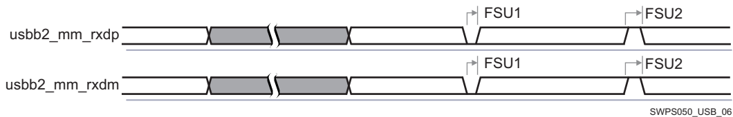
Figure 6-64. Low- and Full-Speed USB—Unidirectional TLL 2-pin Mode—1.8 V
