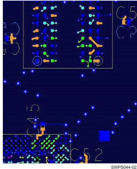
Figure 7-62. Routing DQ0/2 (L1)
