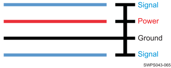
Figure 7-20. Guard Ring Routing
