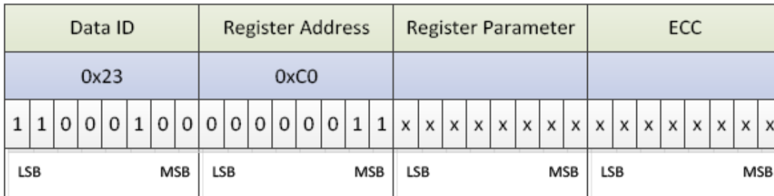
Figure 7–2: Transmission of first capability exchange byte using DSI generic short write packet
